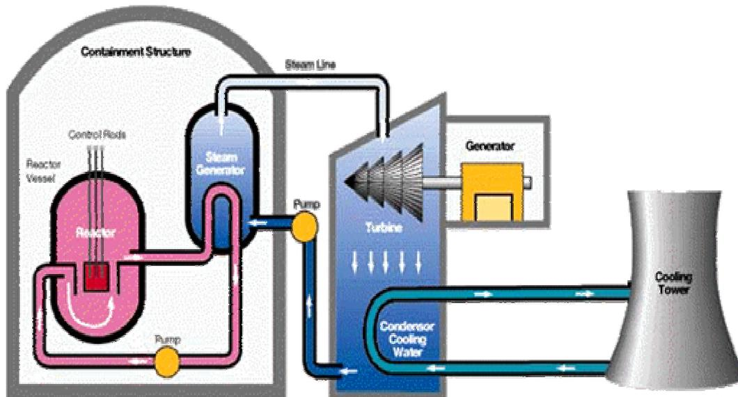
Like all industrial processes, nuclear power generation has **by-product wastes**: spent (used) fuels, other radioactive waste, and heat. Because nuclear generated electricity does not emit carbon dioxide into the atmosphere, nuclear power plants prevent emissions of millions of metric tons of carbon dioxide.
