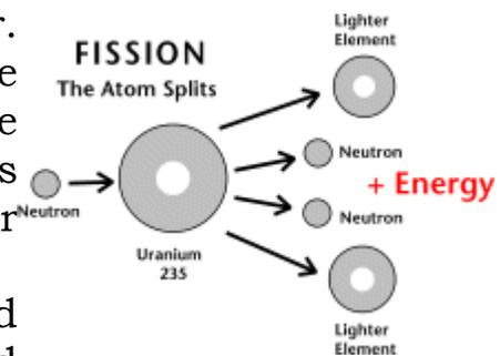
During nuclear fission, a small particle called a neutron hits the uranium atom and it splits, releasing a great amount of energy as heat and radiation. More neutrons are also released. These neutrons go on to bombard other uranium atoms, and the process repeats itself over and over again. This is called a chain reaction.
